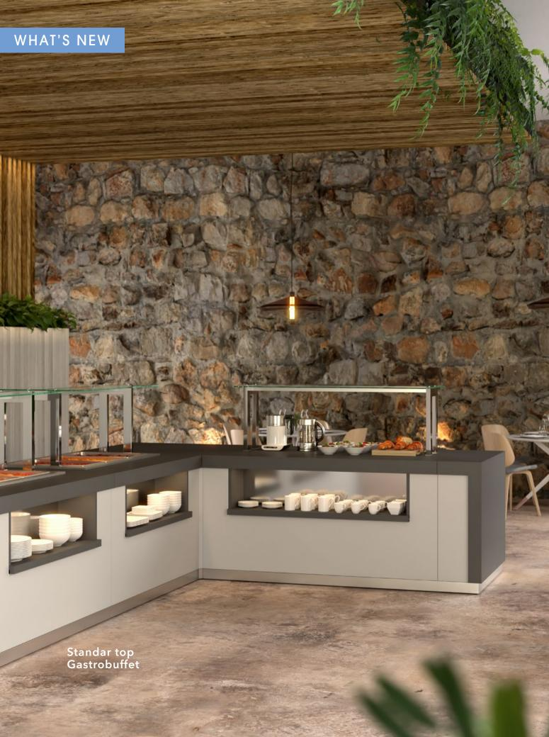
The Gastrobuffet range is the definitive solution for the conservation and display of cold products or beverages. With an automatic defrost system, the temperature control is by means of a digital system. Likewise, the Gastrobuffet range also includes models for preserving hot food.
